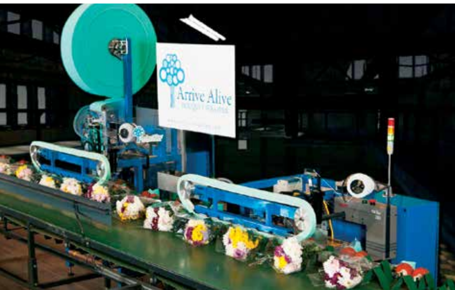
The Arrive Alive® Bouquet Wrapper wraps bouquets at a minimum of 15 to 20 per minute.
